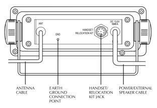
Figure 4-1 Rear Connections
